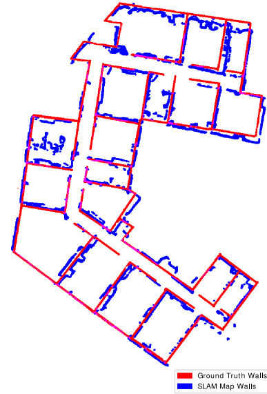
Fig. 5. Office floor 2 : Overlay between the generated SLAM map and its ground truth for a 570 \text{ m}^2 office floor
